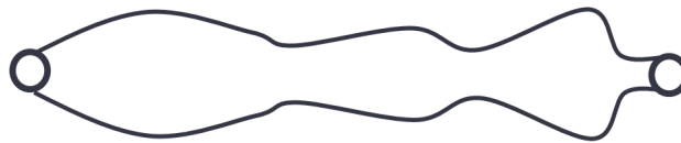
Figure 9.4: The physical analogy of LPC: a tube with varying cross-section.
