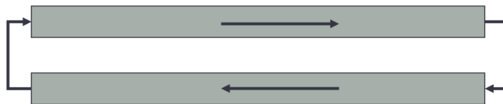
Figure 4: A waveguide model. The right-going and left-going wave, which are superimposed on a single string, are modeled separately as simple delays. The signal connections at the ends of the delays represent reflections. A waveguide can also model a column of air as in a flute.
